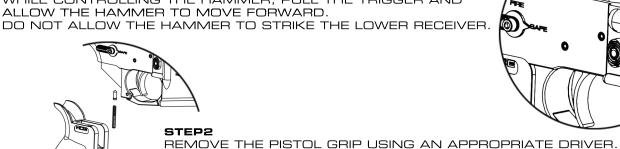
REMOVE THE SAFETY DETENT & SPRING.
